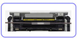
Make sure that the splice area is placed in the middle of the protection sleeve.
