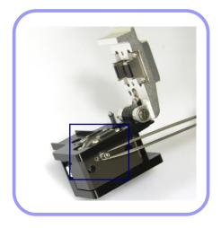
4 Be careful not to damage the blade. Assemble the part in the reverse manner. Tighten the set-screw firmly.
