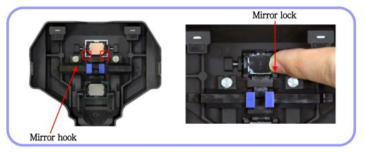
Insert a new mirror into the mirror lock and assemble the parts in reverse manner of disassembling.
