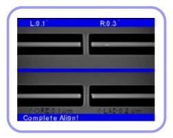
is bigger than the preset limit value or any damage to the fiber is discovered, an error message appears on the screen and the splice process stops. If no error message appears on the screen, examine the condition of the cross sections with your eyes based on following figures. Any fiber that has similar condition to any of below figures has to be removed and a new fiber must be placed. These general defects can cause a wrong splice.
