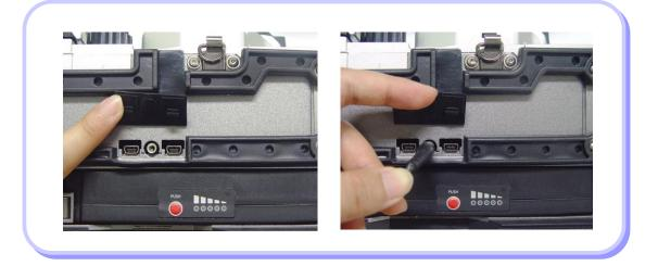
The battery pack includes the protection circuit so that over discharge and over charge can be prevented. The supply of power stops once the protection circuit is activated. In order to deactivate the protection circuit and resume feeding power, wait about 10 seconds and connect the DC plug to the DC jack of the battery pack and the AC cord of the charger to a wall outlet.
