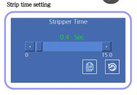
Strip time can be set from 0 to 15 seconds. Select a time frame suitable for the sheath of the fiber to be used.
