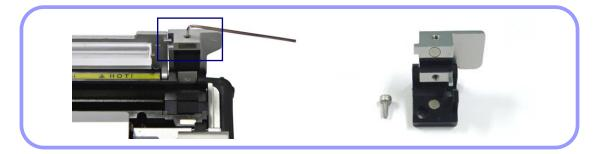
3 Disassemble and replace the Lever Block of left/right side with wrench as picture, as to fiber type.
