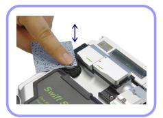
If no alcohol is discharged, open cap and refill the dispenser.Add alcohol after completely removing it from the R5 body by pulling upward. It is connected to the body by magnet.
