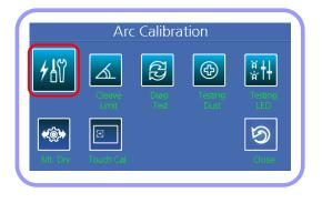
□ [Discharge calibration] is a function to change the "element" value of the discharged voltage. The value is used for the computation program for splicing. In addition, the calibration value of discharge cannot be changed in the splice mode.
