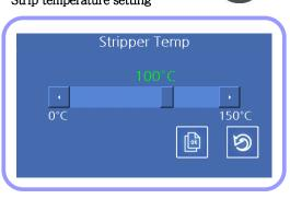
3 Select appropriate strip temperature by using *◄* or *▶* and confirm the adjustment by pressing *◄*.
