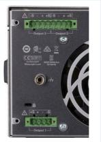
Connections for all channels - including sense lines - are also provided on the rear panel (R&S and Keysight)
