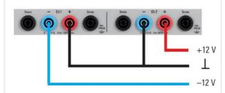
The circuitry of each single channel is completely isolated from the others; there is no connection to chassis ground. This makes it easy to combine the channels to drive balanced circuitries that might need +12 V/-12 V, for example, and avoids ground problems in complex DUTs.
