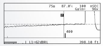
Typical TDR test misses the fault completely.
