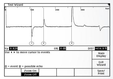
TestWizard<sup>™</sup> Testing automatically marks faults.
