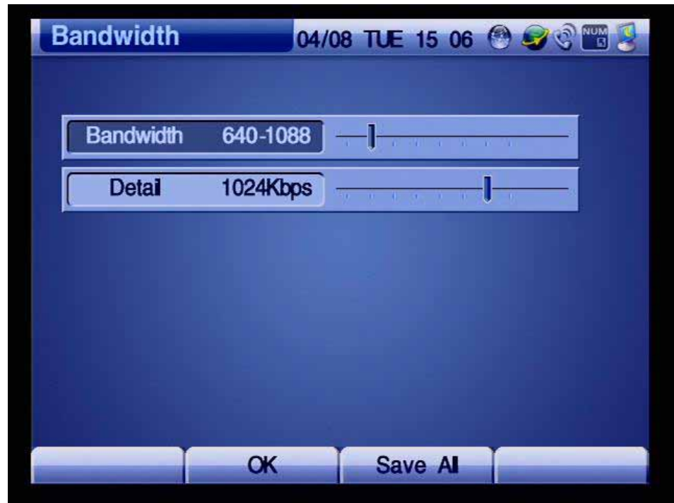
(Figure 4-118) Specifying the Detail option to 1024Kbps and then press F2 to save
