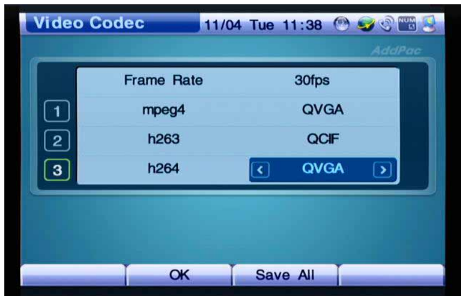
(Figure 4-113) Selecting the Option for the Video Codec of the Third Menu Detail
