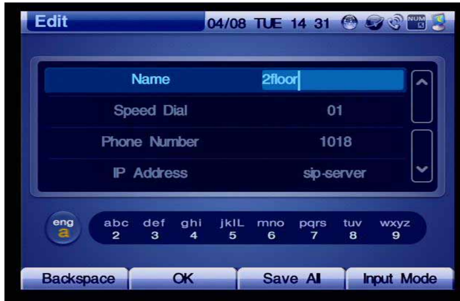
(Figure 4-19) Select Edit Mode by pressing F2 on the remote control
