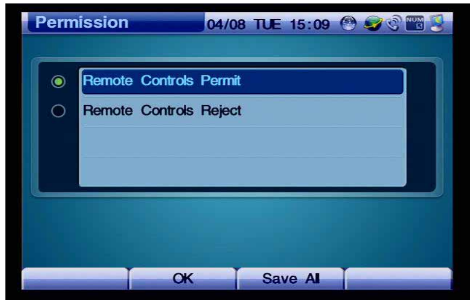
(Figure 4-243) Select the option to permit or reject remote control
