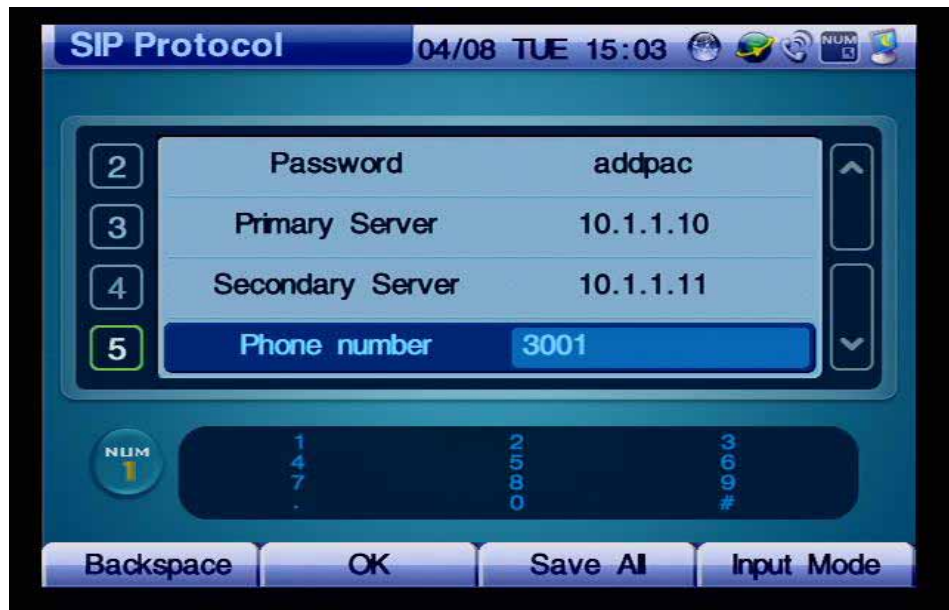
(Figure 4-170) Select the option for setting 'Register E.164' to 'On' and press F2 to save and then enter Phone Number
