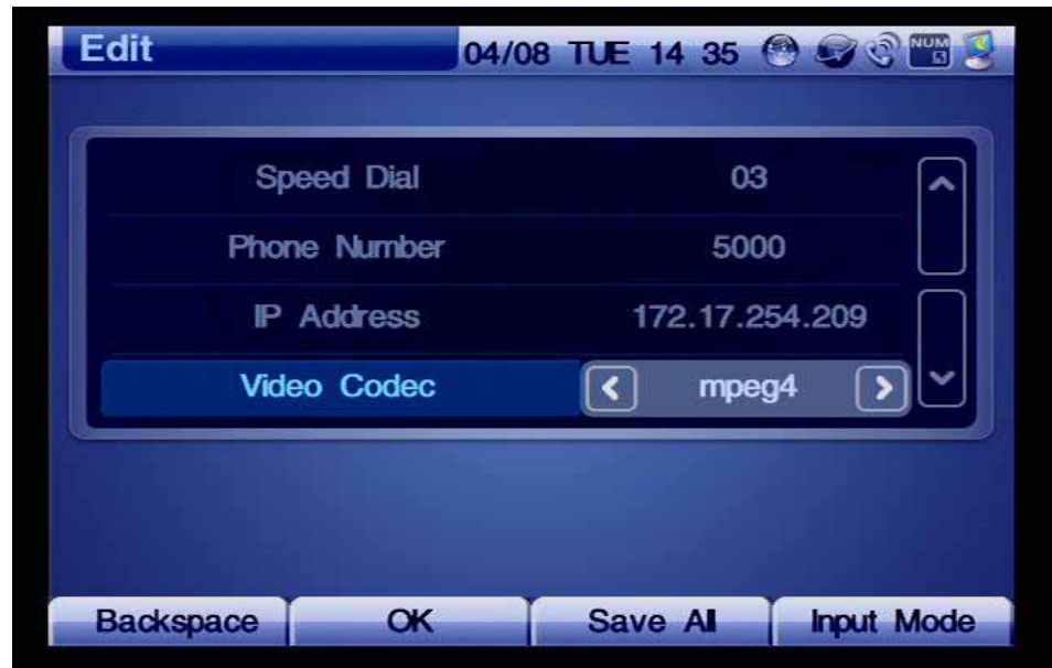
(Figure 4-31) Selecting the Option for Video Codec
