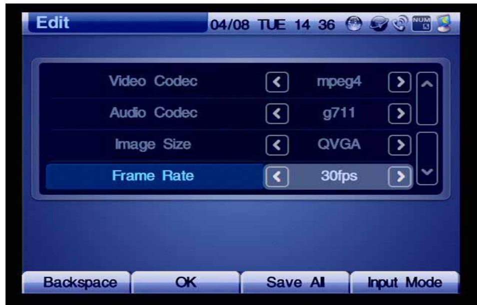
(Figure 4-35) Pressing OK and then Pressing F2 to Save
