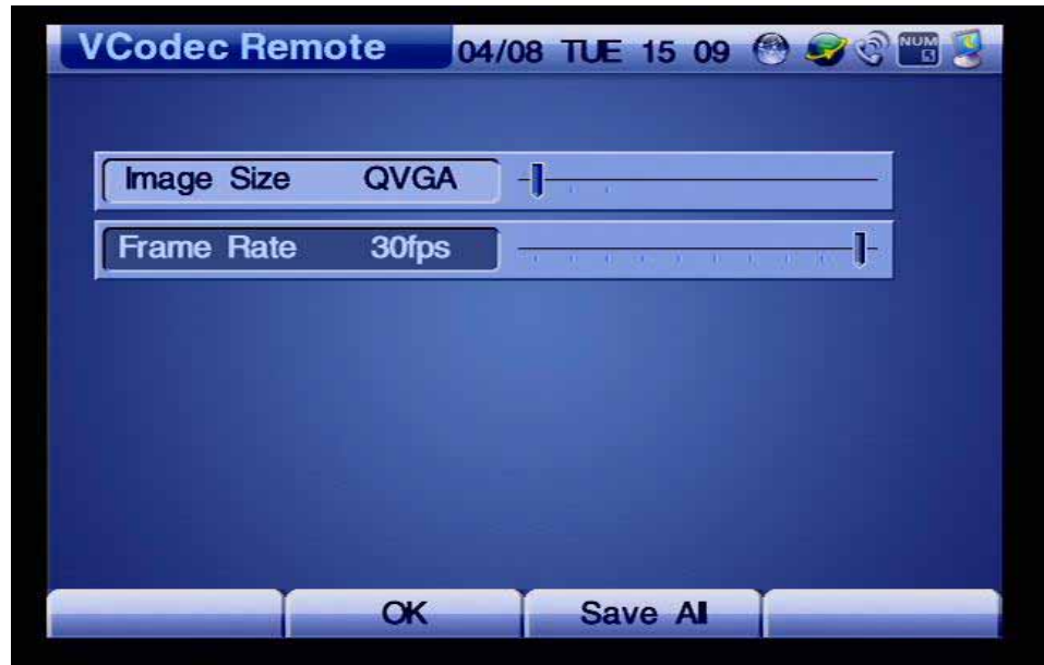
(Figure 4-239) Selecting the Image Size of QVGA at the Frame Rate of 30fps
