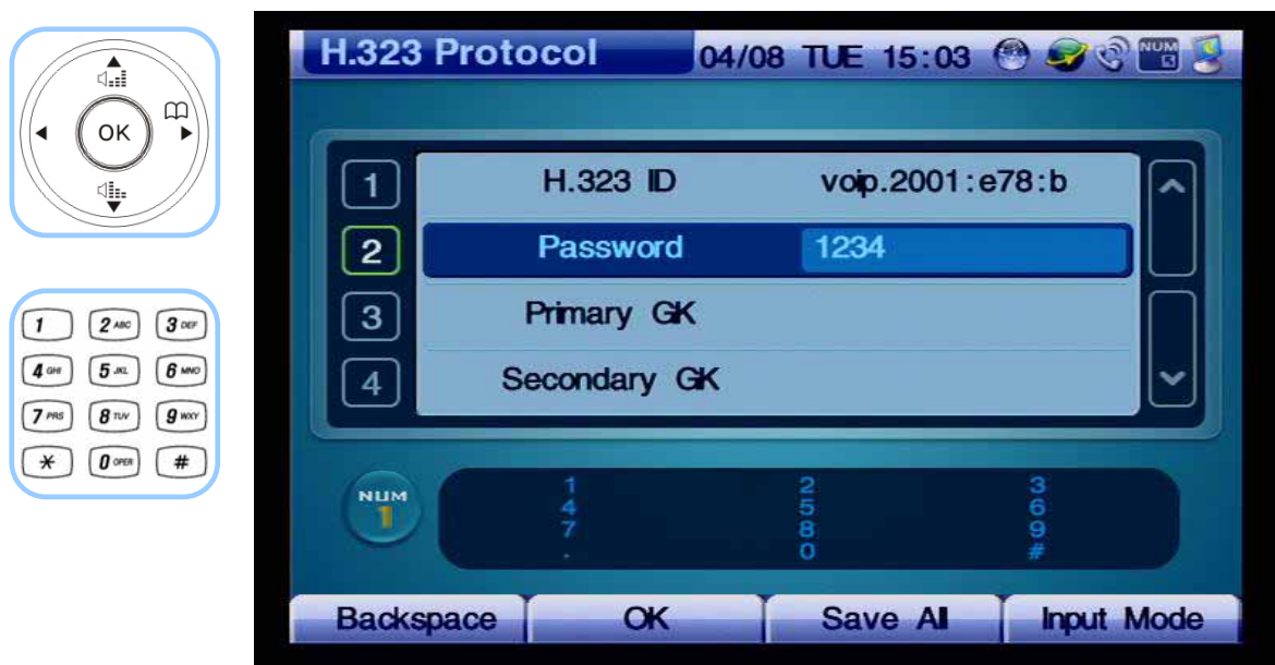
(Figure 4-173) Entering the Password for Registering the Gatekeeper
