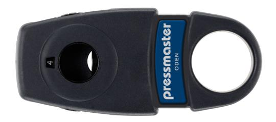
Oden is a precision stripping tool for removing the sheath from signal, telephone, audiovisual, instrumentation and data transmission copper and fiber optic cables. Up to Ø 11 mm/0.43 inch.
