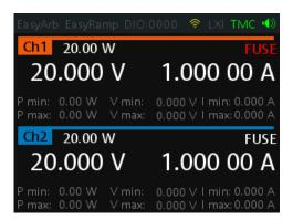
Figure 6-6: Fuse indicator on respective channel
