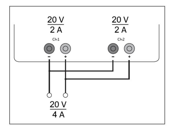
Figure 8-2: Example of parallel connection
