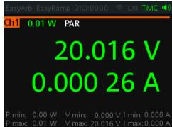
Figure 6-5: Parallel mode setting and output of one-channel display
