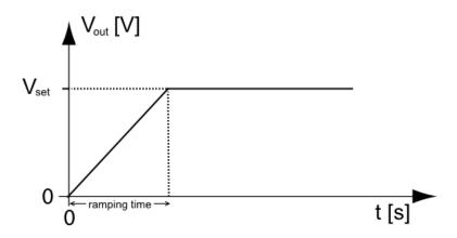
Figure 6-13: Ramping voltage output
