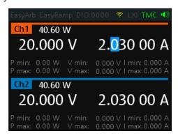
Figure 6-2: Voltage and current settings in the instrument
