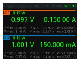
If output current has exceeded 200 mA when current range is set "Low", the "OVLD" information is displayed.
