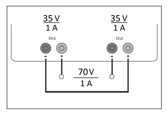
Figure 8-1: Example of series connection
