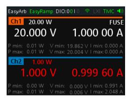
Figure 6-3: Output of Ch2 in CC mode
