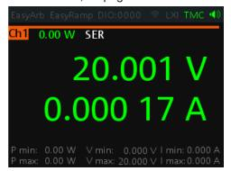
Figure 6-4: Series mode setting and output of one-channel display
