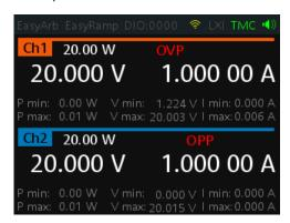
Figure 6-8: Indicator of OVP/OPP when tripped
