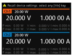
2. Press any of the memory keys ([M1],[M2], [M3], [M4], [M5]) to recall the instrument settings.
