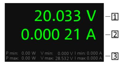
Figure 5-2: Channel display area for one-channel model
