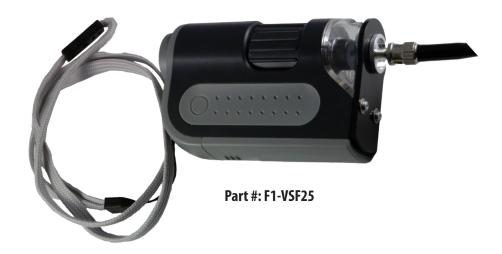
Our fiber inspection scope provides a crystal clear view of both the cladding and core of a ber connector endface to locate defects or contamination. Our standard scope includes a universal 2.5mm adapter that accepts SC, ST or FC connectors in either an APC or UPC configuration.
