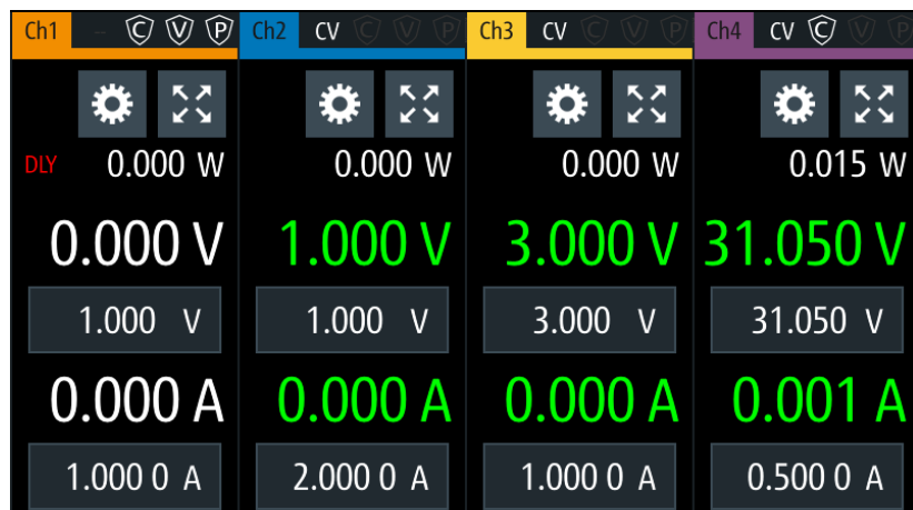
Figure 6-4: Delay text at channel display area
