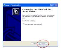
At the Completing the FiberChekPRO Setup Wizard, click Finish to complete software and driver installation.
