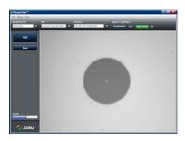
Adjust the focus of the fiber end face image on the computer screen by turning the Focus Control on the microscope.
