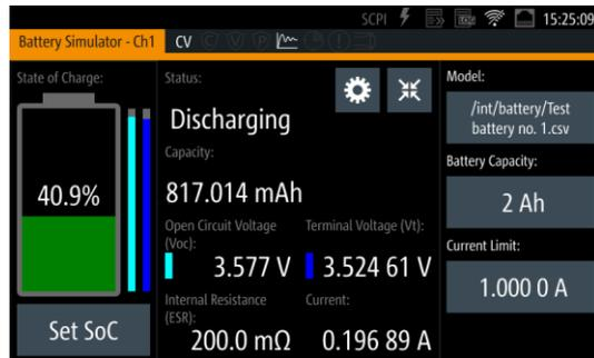
Capacity, open circuit voltage (Voc) and equivalent series resistance (ESR) are important battery characteristics that depend on the battery's state of charge (SoC). The optional R&S®NGM-K106 battery simulator allows users to simulate the battery behavior under different charging conditions, e.g. when powering a DUT.
