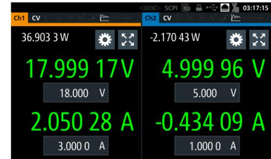
A resolution of up to 6½ digits is perfect for characterizing DUTs that have low power consumption in standby mode and high current in full load operation.
