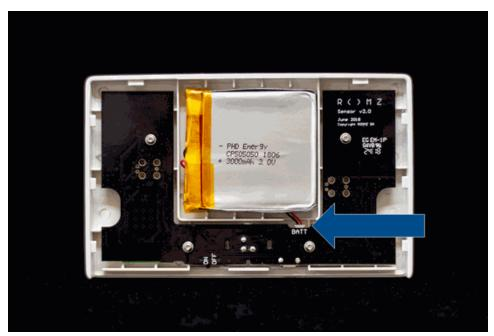
• Remove the sticker's sleeve, plug the new battery in, and stick the battery back in place
