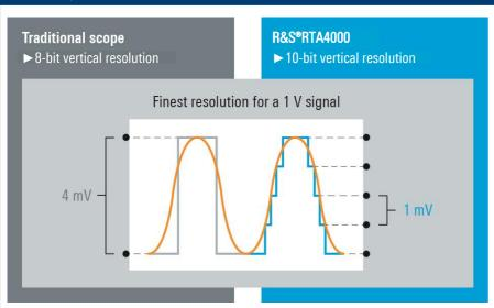
The R&S®RTA4000 features a customized Rohde & Schwarz 10-bit A/D converter that delivers a fourfold improvement over conventional 8-bit A/D converters.
