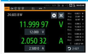
The large capacitive touchscreen is the central operating element. With its very high resolution of  $800 \times 480$  pixel, the display makes it easy to read the voltage and current fields even at great distances. Additionally, information such as power values or statistics can be displayed. Icons clearly show the status of the set protection or special functions.
