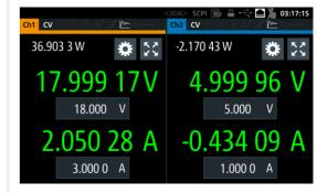
A resolution of up to 6  $\frac{1}{2}$  digits is perfect for characterizing DUTs that have low power consumption in standby mode and high current in full load operation. The R&S\*NGL200 power supplies automatically switch from source to sink mode. Operating as a load is indicated by a negative current reading.
