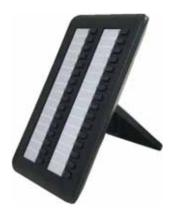
A maximum of four DSS532 can be attached to EON510/SPARSH VP510. With each DSS532, 32 additional keys are at your disposal to be used as DSS keys. Similarly, if four DSS532 are attached, 128 additional keys are at your disposal to be used as DSS keys.
