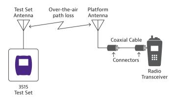
VIAVI Solutions understands that in today's market digital communications are just as important as voice communications. The 3515 verifies digital radios over-the-air and non-intrusively. The 3515 supports EPLRS, SADL, and P25 radios.
