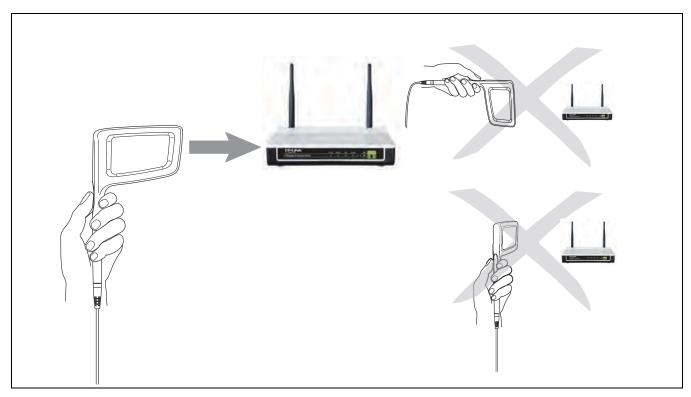
Figure 56. How to Point the External Antenna
