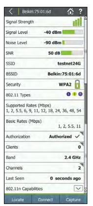
Figure 9. Access Point Details Screen
