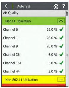
Figure 20. 802.11 Channel Utilization Results
