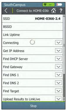
Figure 44. The Connect to Network Test (In Progress)
