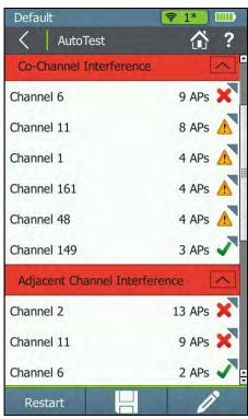
Figure 22. Air Quality Co-Channel and Adjacent Channel Interference Results
