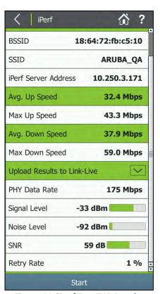
Figure 64. iPerf Test TCP Results
