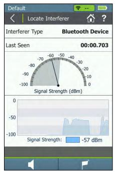
Figure 54. Locate Interferer Screen
