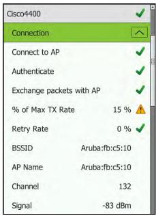
Figure 27. AutoTest Network Connection Test Results
