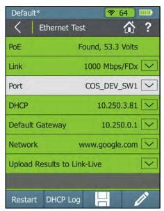
Figure 32. Ethernet Test Screen
