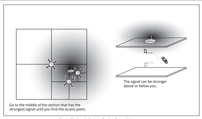
Figure 55. Search Pattern for the External Antenna
