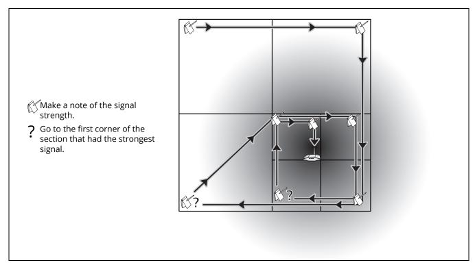
Figure 50. Search Pattern for the Omni-directional Antennas in the Tester
