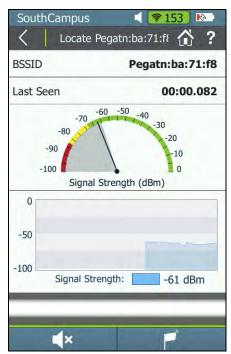
Figure 51. Locate Access Point Screen
