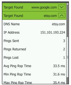
Figure 48. Connection Test Target Results
