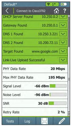
Figure 47. Connect to AP Test Results Continued
