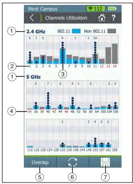
Figure 10. Channels Utilization Screen
