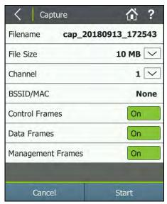
Figure 66. Capture Screen (Setup)
