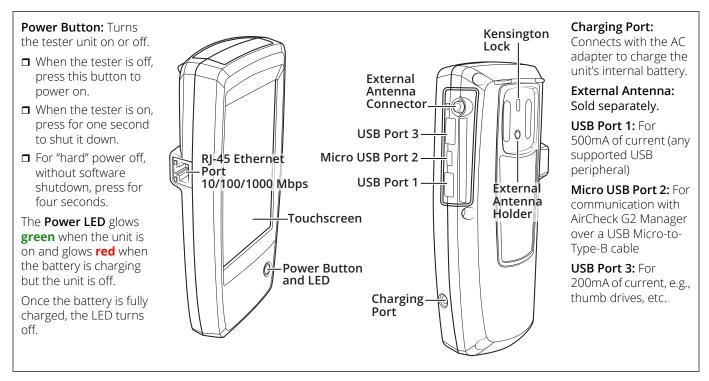
Figure 1. AirCheck G2 Physical Features
