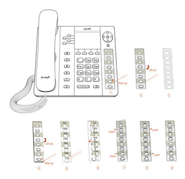
Step1. Use needle or some other tools to insert into the hole of the plastic sheet, hog the plastic sheet.
