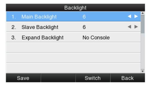
To adjust the brightness of LCD expansion module, it must be connected with the hosted phone. Otherwise the host phone will indicated "No expansion module".
