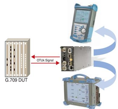
Transport Blazer modules support G.709 testing in either the FTB-200 Compact Platform or the FTB-400 Universal Test System.
