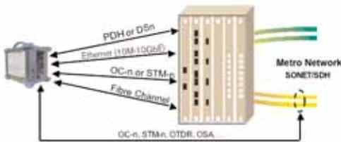
With its modular, multislot design, the FTB-400 platform enables users to configure and upgrade their systems in the field according to their testing needs, minimizing capital expenditures.
