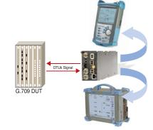
Transport Blazer modules support G.709 testing in either the FTB-200 Compact Platform or the FTB-400 Universal Test System.
