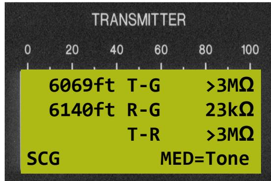
R-G Ohms has come down from the 154k Ohms to **23k Ohms** since the capacitance of the crossed pair(s) has been cancelled (grounded) out.
