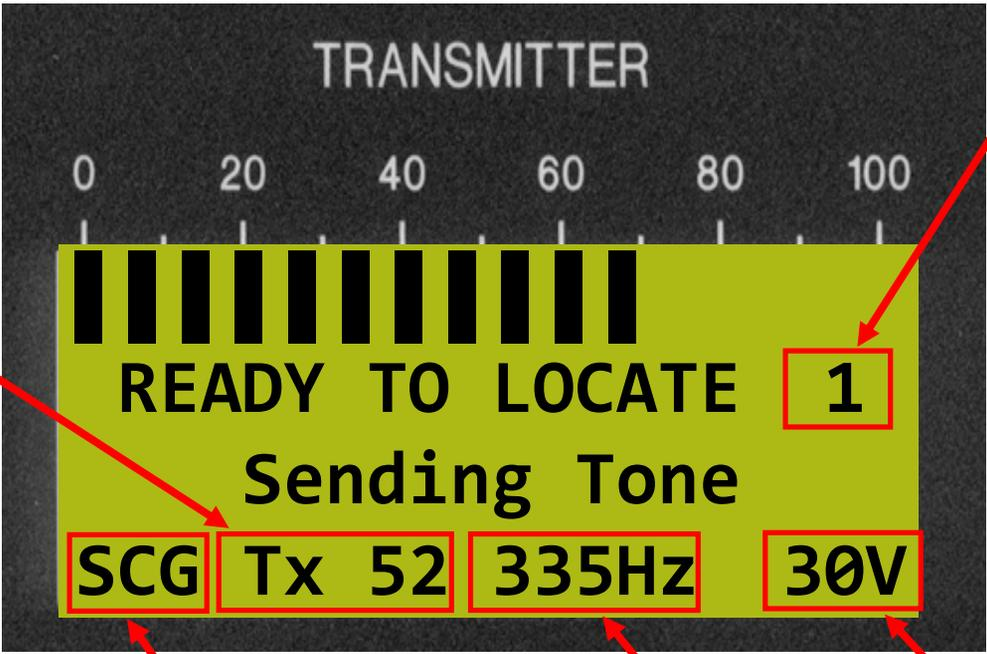
This Length Ratio number indicates the likelihood of tone carry-by. Chance for a successful locate is excellent when length ratio is 1, under 10 is good, the lower the better.
