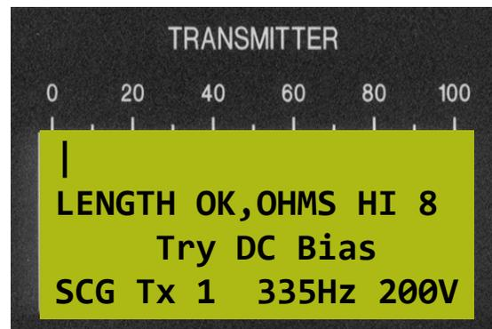
When a high resistance fault will not produce adequate tone for tracing, the DC BIAS will dislodge any insulating oxide layer present to bring faults **up to 1M Ohm** down into the Locatable Fault Range, especially in PIC cable.
