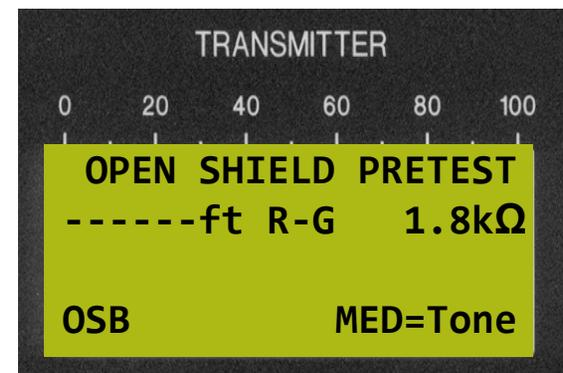
**If the R-G length is dashed out you cannot get an estimated distance to the fault, continue toning the fault.**
