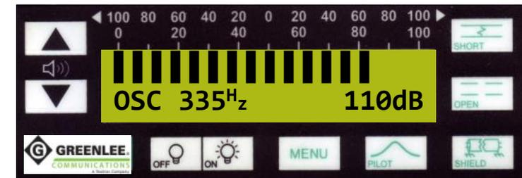
**CAUTION: When toning an Open Shield in Coil mode only, do not touch the back panel of the Receiver as it may ground out the tone!**
