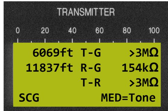
R-G Ohms indicates the unbalance is **not** a one sided open. The 154k Ohms is an AC Ohms indication and will not be the same as your DC Ohmmeter until the pairs you are crossed with are identified and grounded.
