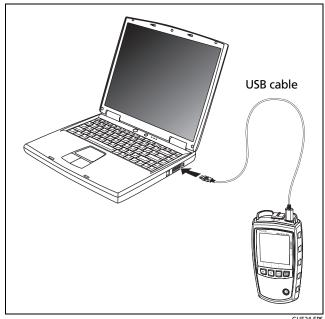
Figure 12. Connecting to a PC
