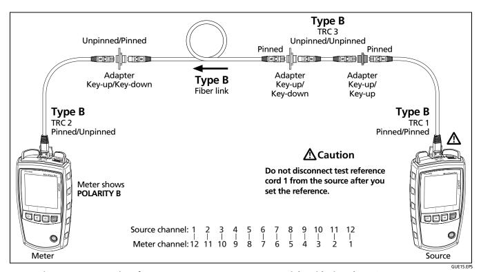
Figure B-13. Connections for Loss Measurements on Permanent Links with Pinned MTP/MPO Connectors when Links are Used with Corning Plug & Play™ Universal Systems
