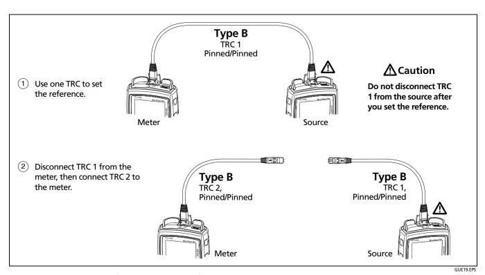
Figure B-1. Reference Connections for Permanent Links with Unpinned MTP/MPO Connectors
