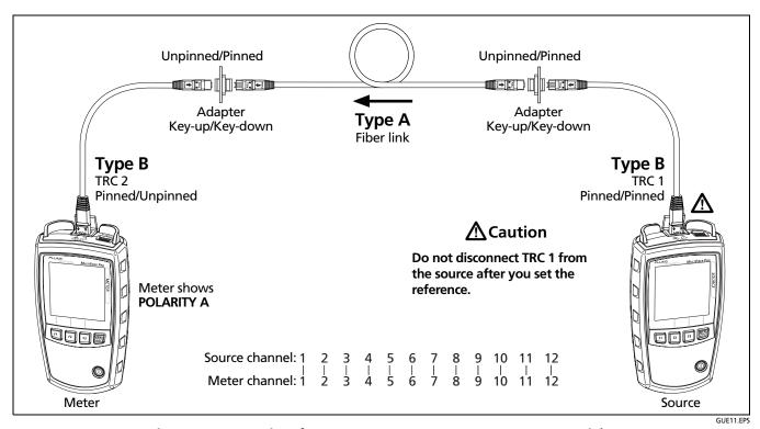
Figure B-6. Connections for Loss Measurements on Type A Permanent Links with Unpinned and Pinned MTP/MPO Connectors
