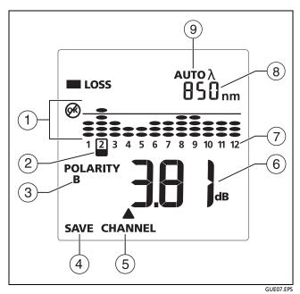
Figure 10. Loss Measurement Display
