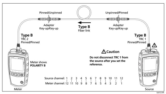
Figure B-3. Connections for Loss Measurements on Type B Permanent Links with Unpinned MTP/MPO Connectors
