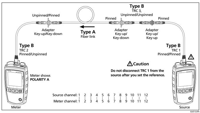
Figure B-10. Connections for Loss Measurements on Type A Permanent Links with Pinned MTP/MPO Connectors
