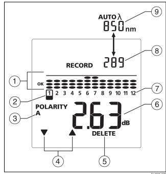
Figure 11. View Record Display (loss measurement shown)
