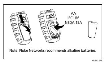
Figure 1. Installing the Batteries
