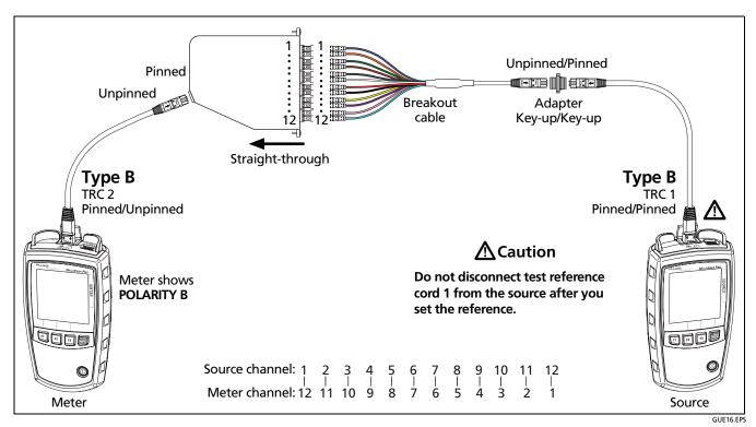
Figure B-15. Connections for Loss Measurements on a Straight-Through Fiber Module with a Pinned MTP/MPO Connector
