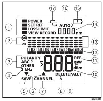
Figure 3. Meter Display Features
