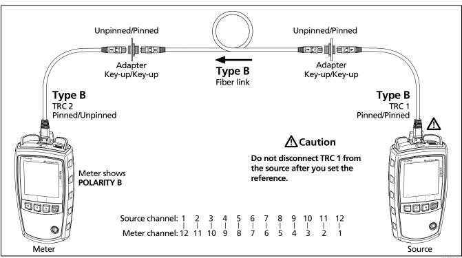
Figure B-7. Connections for Loss Measurements on Type B Permanent Links with Unpinned and Pinned MTP/MPO Connectors
