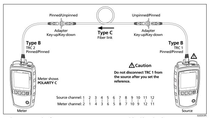
Figure B-4. Connections for Loss Measurements on Type C Permanent Links with Unpinned MTP/MPO Connectors
