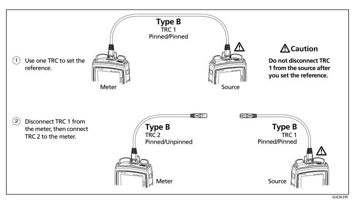
Figure B-5. Reference Connections for Permanent Links with Pinned and Unpinned MTP/MPO Connectors
