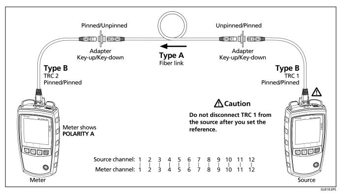
Figure 9. Connections for Loss Measurements on Type A Permanent Links with Unpinned MTP/MPO Connectors
