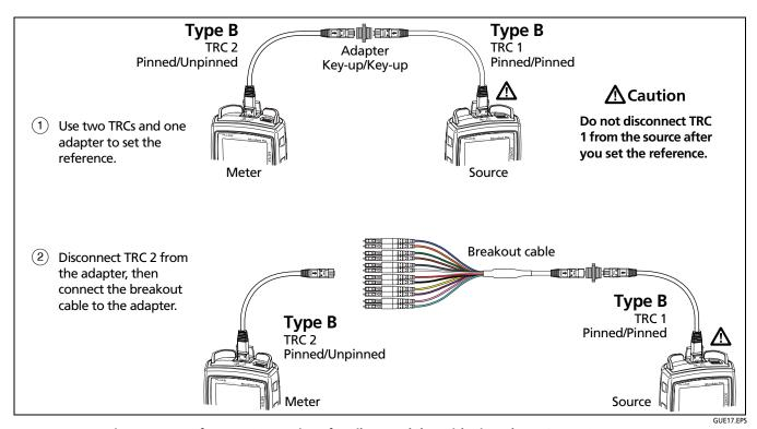
Figure B-14. Reference Connections for Fiber Modules with Pinned MTP/MPO Connectors
