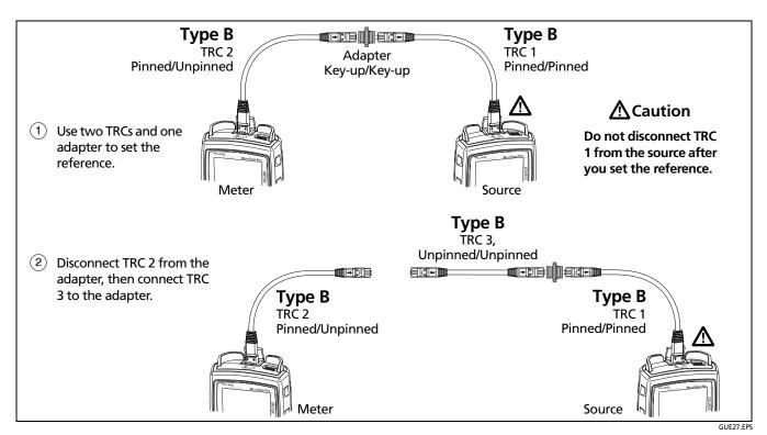
Figure B-9. Reference Connections for Permanent Links with Pinned MTP/MPO Connectors
