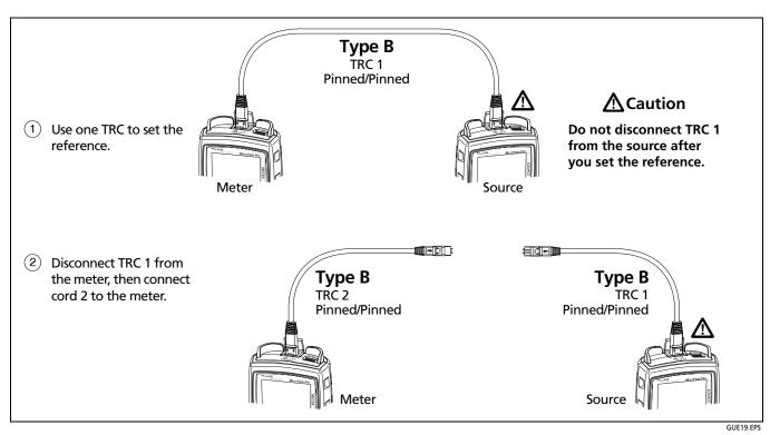
Figure 8. Reference Connections for Permanent Links with Unpinned MTP/MPO Connectors
