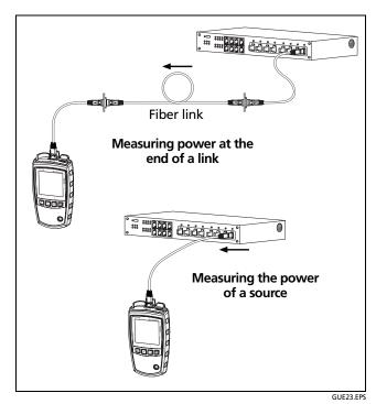
**Figure 6. Connections for Power Measurements**
