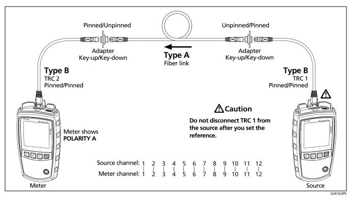
Figure B-2. Connections for Loss Measurements on Type A Permanent Links with Unpinned MTP/MPO Connectors
