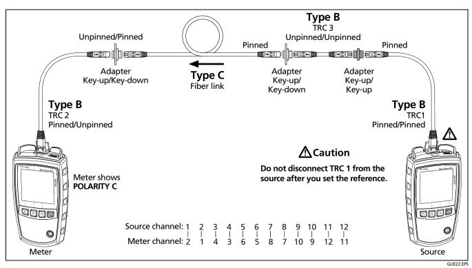
Figure B-12. Connections Loss Measurements on Type C Permanent Links with Pinned MTP/MPO Connectors
