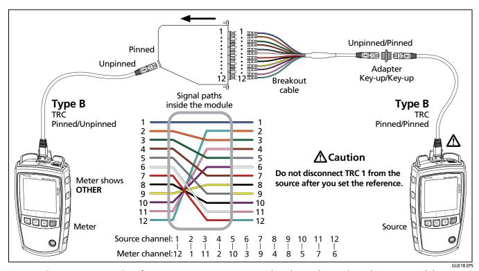
Figure B-16. Connections for Loss Measurements on a Corning Plug & Play™ Universal Systems Module
