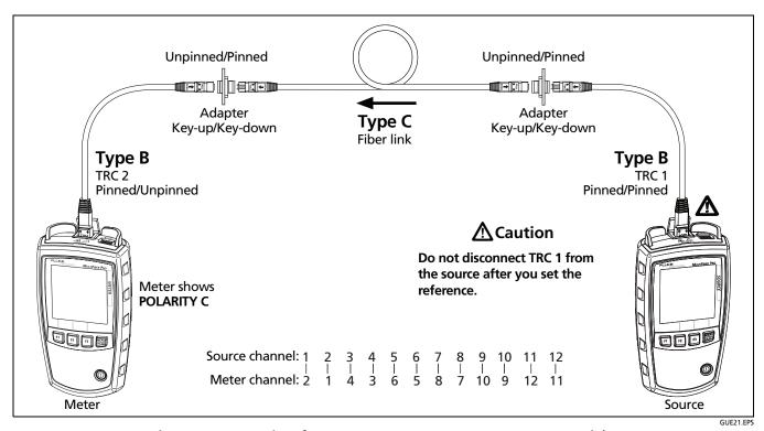
Figure B-8. Connections for Loss Measurements on Type C Permanent Links with Unpinned and Pinned MTP/MPO Connectors
