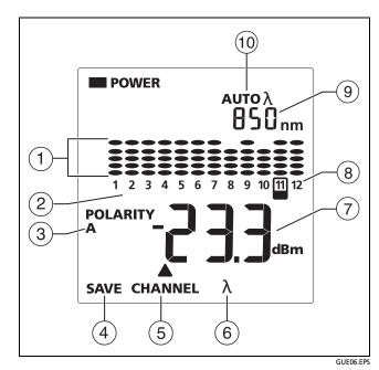
Figure 7. Power Measurement Display
