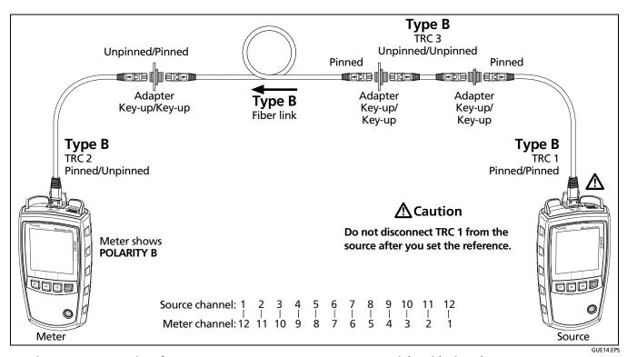
Figure B-11. Connections for Loss Measurements on Type B Permanent Links with Pinned MTP/MPO Connectors
