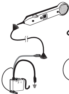
Figure 4a. Cable Tracing
