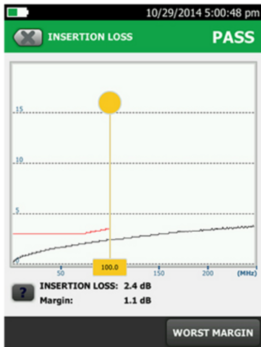
Figure 1. Measured Insertion Loss and limit for 100 foot Type 734 cable.
