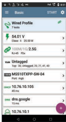
NBASE-T network with VLAN and 802.1x authentication
