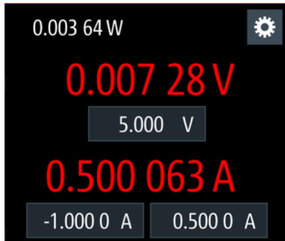
Figure 6-2: Output of R&S NGU in CC mode
