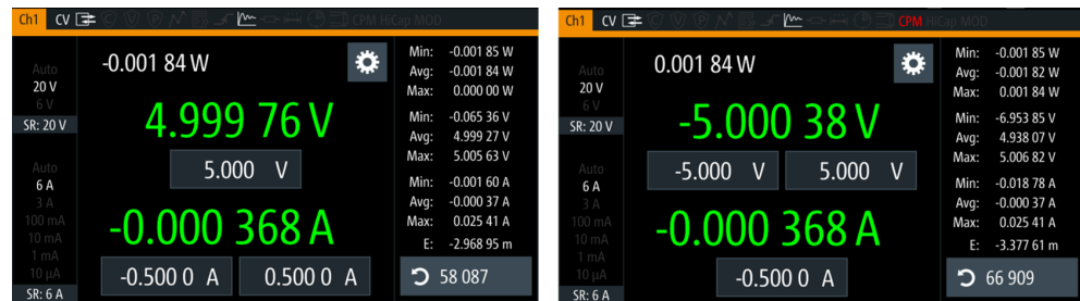
Figure 6-9: NGU401 model switches from VPM to CPM
