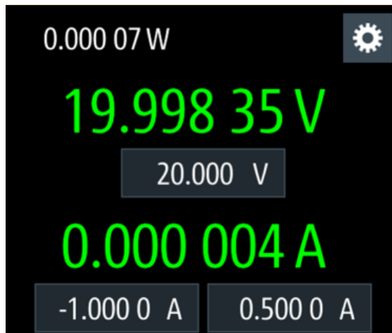
Figure 6-1: Voltage and current settings in the instrument
