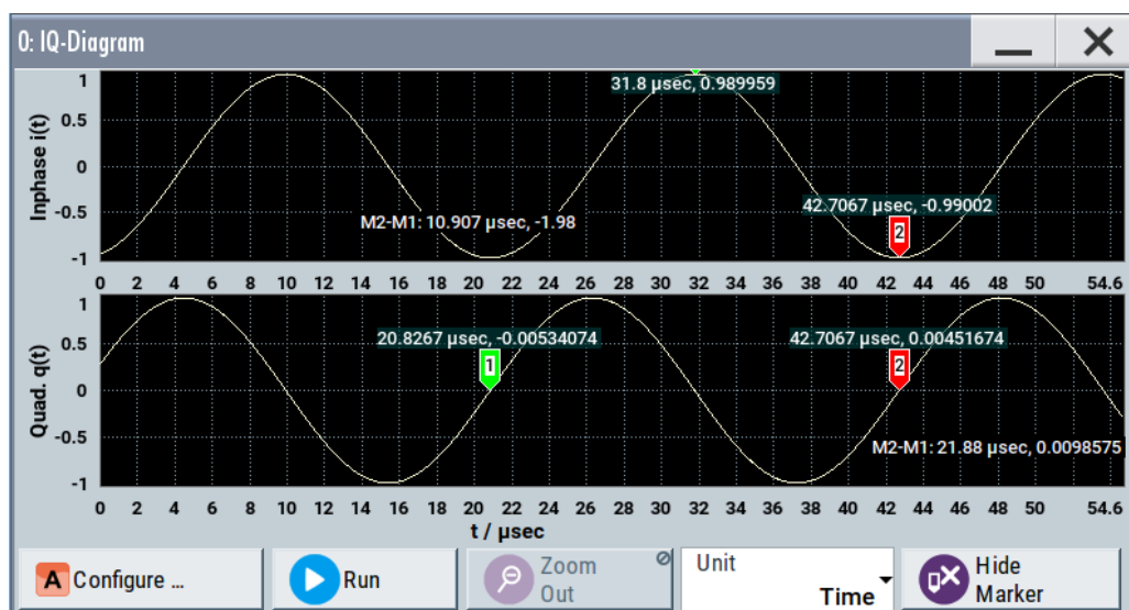
Figure 9-1: I/Q diagram with markers
