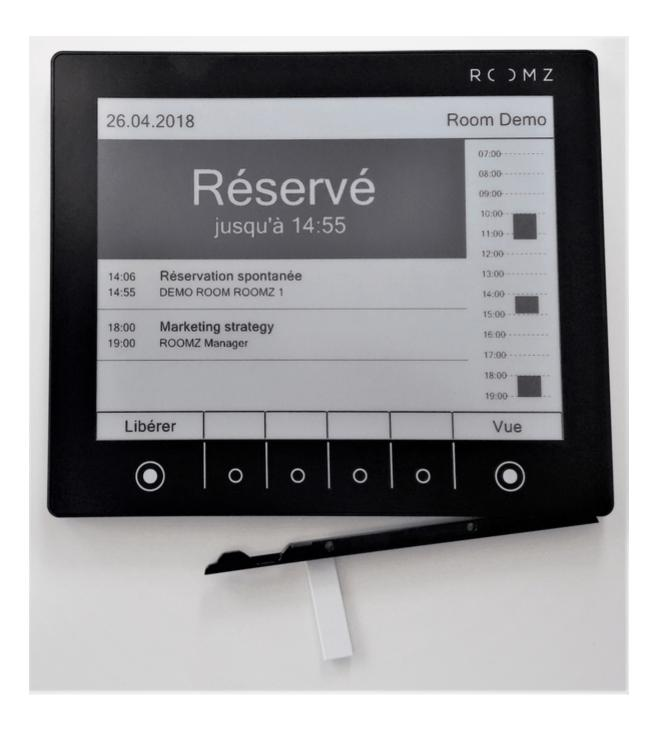
• Using a paperclip, unfold the strips sticking on the battery, that will help you slide the battery out:
