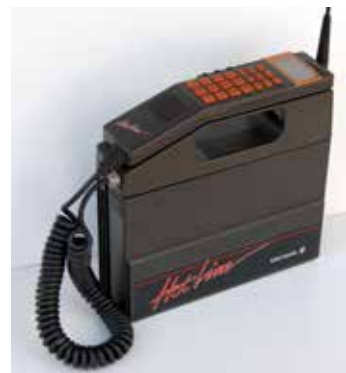
The first ‘portable’ Hotline Ericsson weighed 3.5 kg and cost around 30 000 SEK in the end of the 1980s.
