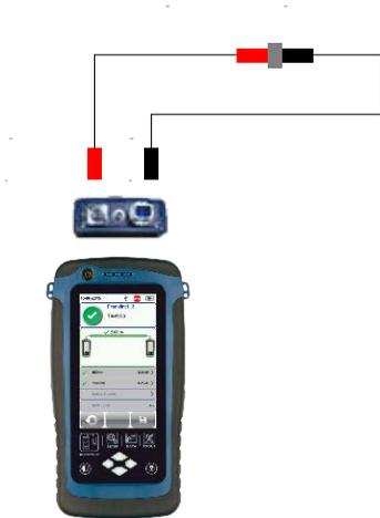
3. Press the SETUP button > Configuration and select “Two Jumper” from Single-Ended column. Select Single or Bi direction depending on requirement.
