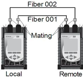
6. To begin the AutoTest sequence, press the AutoTest button on the unit. Leave Remote unit in the Startup screen.
