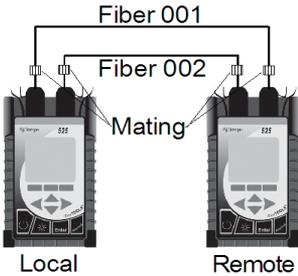
10. Reverse the fiber connections. Perform this at the mating – do not reverse the reference cables at the unit itself.
