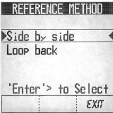
From the Autotest Main screen, press the REF softkey. The Reference Method screen will be displayed. Use the UP/DOWN arrow keys to highlight ► SIDE BY SIDE ◀ or ► LOOP BACK ◀.
