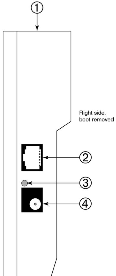
4. DC input receptacle: The power transformer/NiMH battery charger is connected to this receptacle.
