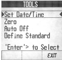
From the Menu screen, use the UP/DOWN arrow keys to highlight the ►TOOLS◀ function, then press the Enter button to select. Use the UP/DOWN arrow keys to highlight the function, then press the Enter button to select and modify the following:
