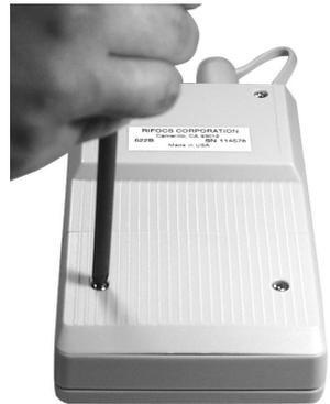
Installation of the battery cover is the reverse of removal. Take care not to overtighten the screws securing the battery cover or damage may result.
