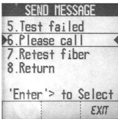
The 525-30 has eight stored messages that can be sent between units when performing Insertion Loss testing. These messages are pre-programmed and cannot be modified by the user -
