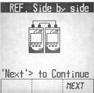
Note: The unit initiating a test or reference is the 'Local' unit, and will hold the references. The other unit is the 'Remote' and should be in this screen.
