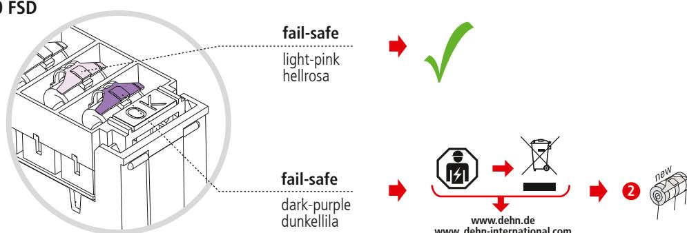
Fig. 6 Test, Measuring / Test, Messung
