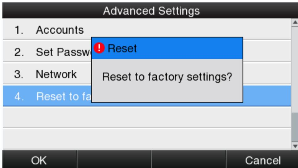
Reset to factory via Web: **Phone** → **Upgrade** → **Reset to Factory**.
