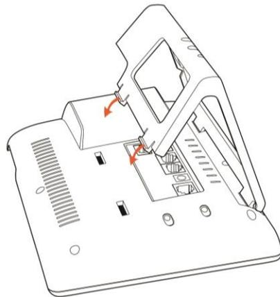
C. It is the right picture after fixing the stand bracket below:
