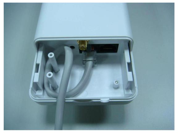
Step3: Install the upper housing and make sure the housing is well installed.
