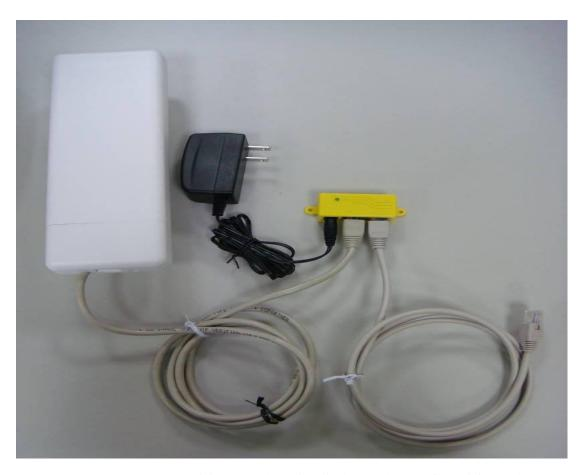
Notes: Use **Reset button** on POE injector. Push continually the reset button of POE injector about  $5 \sim 10$  seconds to reset the configuration parameters to factory defaults.
