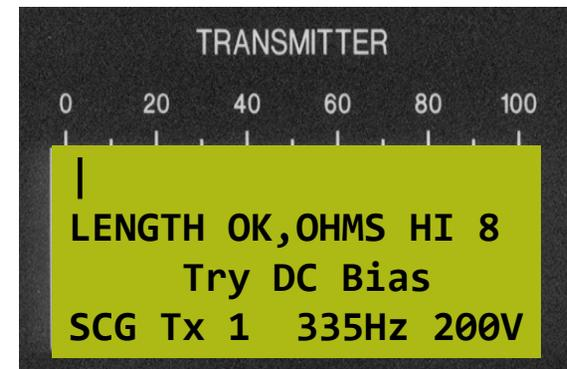
When a high resistance fault will not produce adequate tone for tracing, the DC BIAS will dislodge any insulating oxide layer present to bring faults **up to 1M Ohm** down into the Locatable Fault Range, especially in PIC cable.
