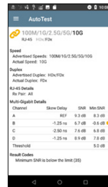
Cabling SNR measurement validates Multi-Gig links
