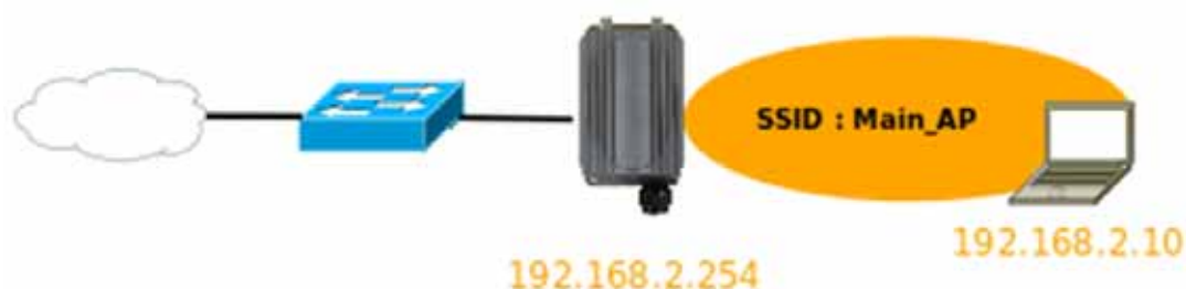
Figure 3-1 Access Point on a Wired LAN Configuration
