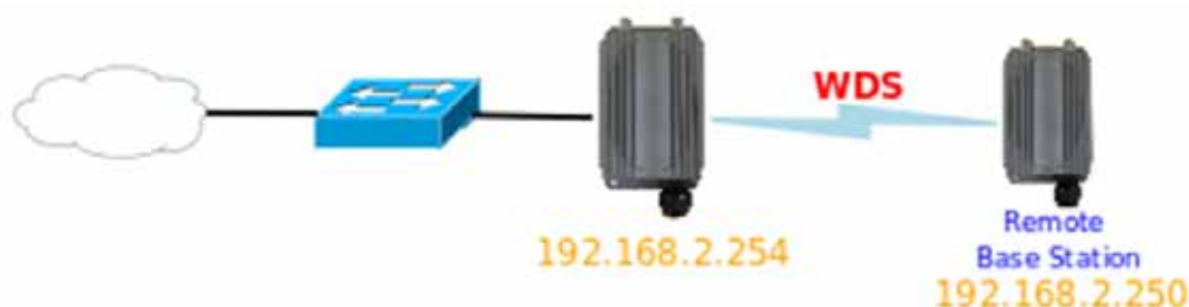
Figure 4-1 Point to Point network Configuration
