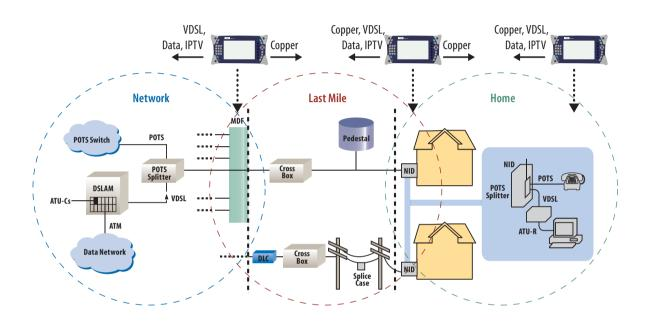
Figure 3: Example of a typical DSL architecture
