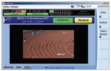
Figure 4: Example of IPTV Video Stream test
