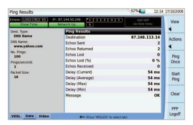
Figure 7: IP Ping test interface
